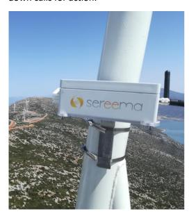
Aware of their needs, Sereema has developed an expert solution to analyze and optimize operations of wind turbines. The so-conceived proprietary system comes in the form of an IoT sensor box, embedding MEMs sensors, equipped directly on the turbine; a stream processing platform with its own algorithms to mull the data over; and a user dedicated website displaying all independent results under useful dashboards.
